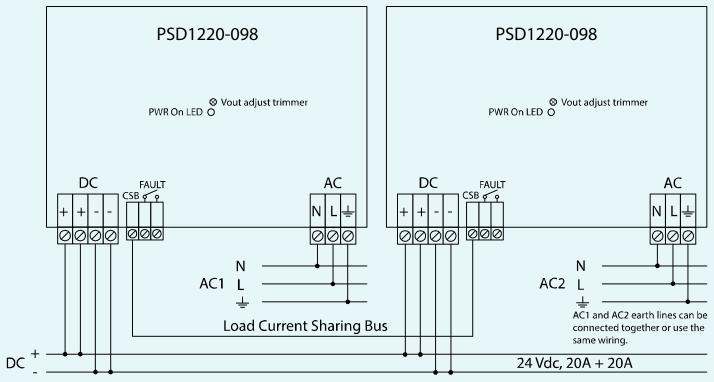
In this application, for each PSD1220-098, double wiring (on positive and negative output poles) is suggested between DC output connector and DC bus.
