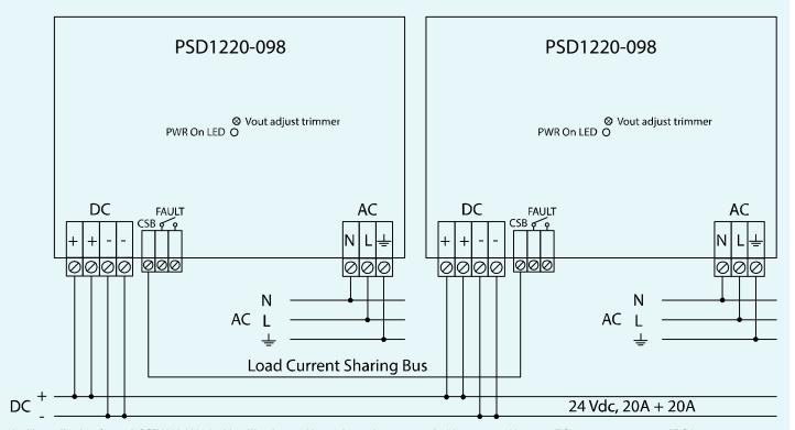
In this application, for each PSD1220-098, double wiring (on positive and negative output poles) is suggested between DC output connector and DC bus.
