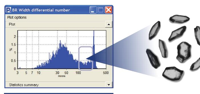
The Particle Insight allows the user to have a true analysis of all dimensions of the particles. In addition, the user is able to selectively see each particle that created a certain area of any shape histogram.
