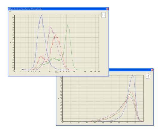
Most particle size analyzers assume particles to be spherical without taking into account other critical shape factors. In the above example, the difference in two samples, similar in size when assumed to be spherical, are clearly demonstrated in overlays of both circularity and smoothness. Only a particle shape analyzer can render such critical shape information.
