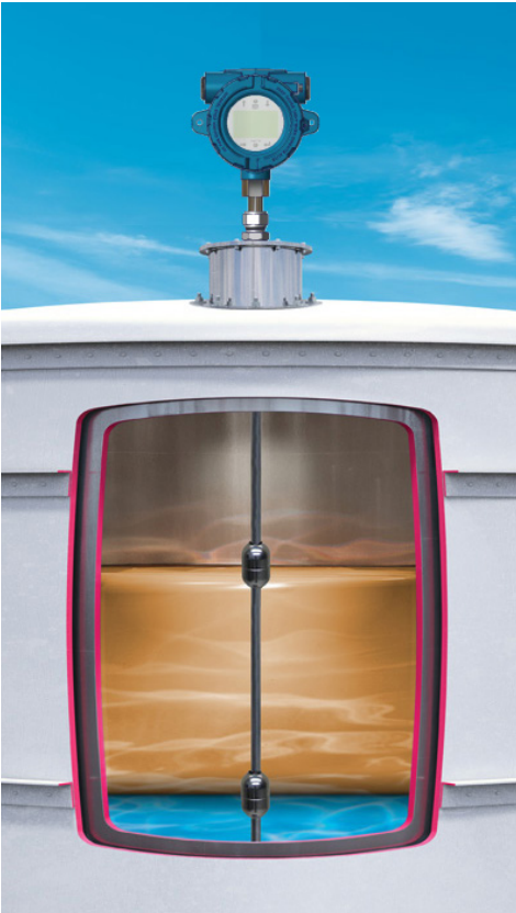
Fig. 2: Example of product and interface level measurement
