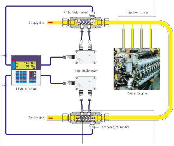
Using temperature sensors, the BEM 4U displays fuel consumption in mass units.
