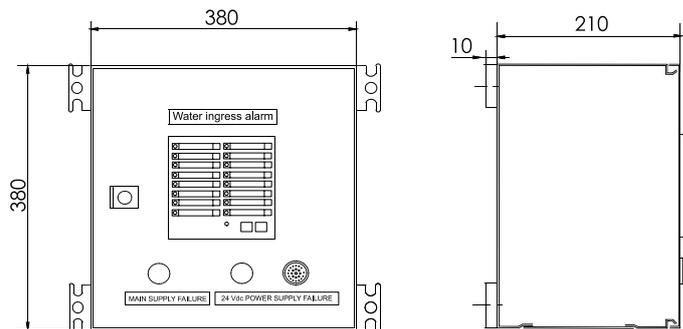
The dimensions can be modified according to the number of alarm units to be supplied
