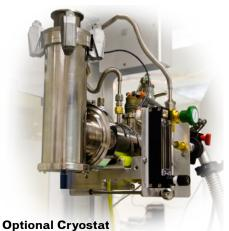
A single-stage cryogenic refrigerator that operates on the Gifford-McMahon refrigeration cycle. It uses helium gas from a helium compressor(s) to offer a wide range of analytical temperatures with milli Kelvin levels of stability.
