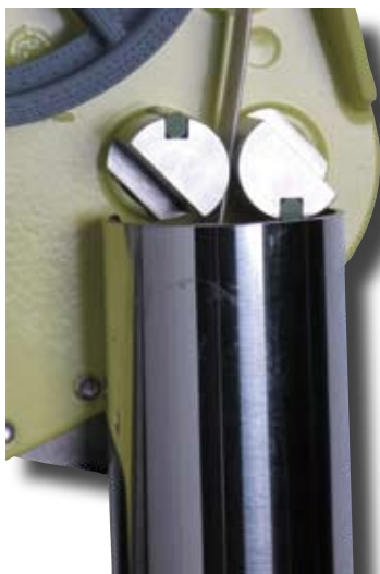
Protection tube to avoid spills and keep working space clean
