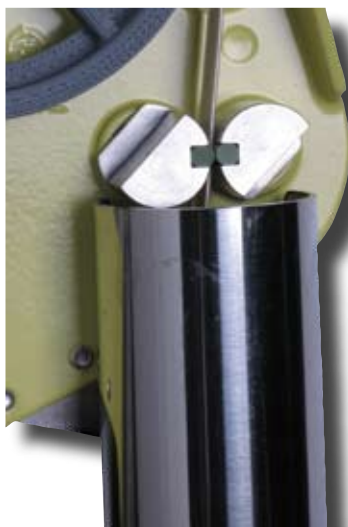
Protection tube to avoid spills and keep working space clean
