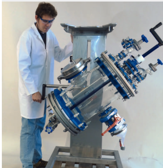
tilting of 30 liter high containment filter vessel for discharge Drehung des 30 Liter high containment Filters für Entladung
