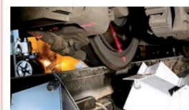
Real Time Wheel Geometry Measurement System, 3DWheel
