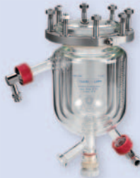
with bottom valve and tripple jacket for low temperature
