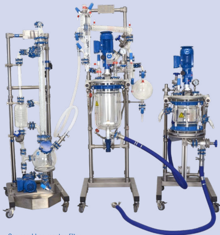
Gas scrubber, reactor, filter Gaswäscher, Reaktor, Filter
